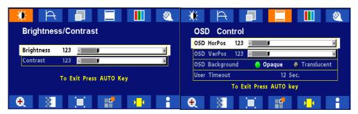
Push "Up" or "Down" button to select between "Brightness" or "Contrast" then push "Select" Use "Left" or "Right" button to adjust Push "Up" or "Down" button to select between "OSD Hor. Pos.", "OSD Ver. Pos.", "OSD Background", or "User Timeout" then push "Select" Use "Left" or "Right" button to adjust
